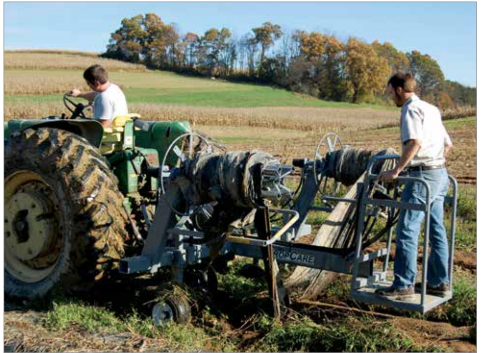
By utilizing film-lifting equipment, farmers can save $125 per year per acre in labor and other costs.
