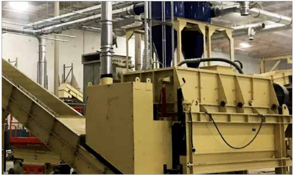
The use of a dry impact separator can reduce dirt levels in recovered ag plastics without water.
