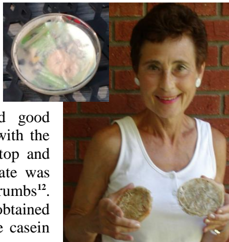
Upper left photo: Casein plastic/paper composite cast in Pyrex form. Lower photo: Casein/crumb rubber composite; casein/shredded milk carton composite
